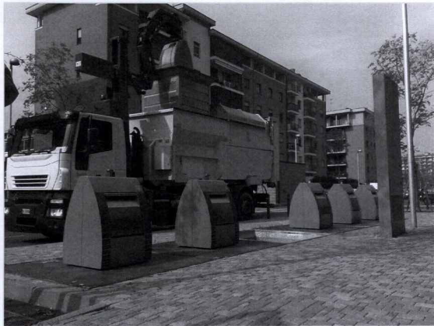
Sample image of Special Compression Garbage Truck With 2 Cranes and Hooking 20m3
